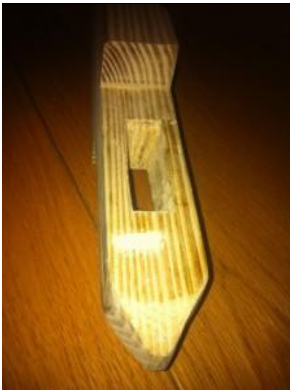
Mortise in the end of a stretcher
