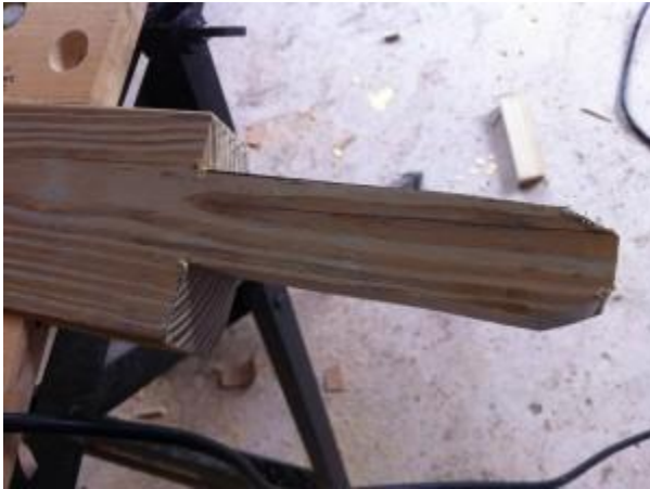
Cutting the ends of the stretchers
